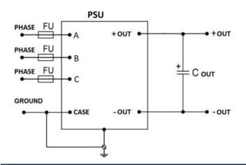
In any system application it's necessary to at least use minimal connection scheme consisting of components shown on the picture.
