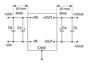
In any system application it's necessary to at least use minimal connection scheme consisting of components shown on the picture.
