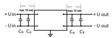
The design of the units allows their use only when mounted on a PCB. When using the units + U out with typical connection scheme it's necessary to use certain type components. In the figure: Ck – - U out ceramic capacitors of a certain operating voltage and of several μF capacity; Ce – electrolytic capacitors of a certain operating voltage and of
