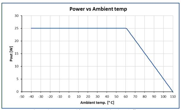
The graph is constructed for a 25 W model with 88% efficiency.
