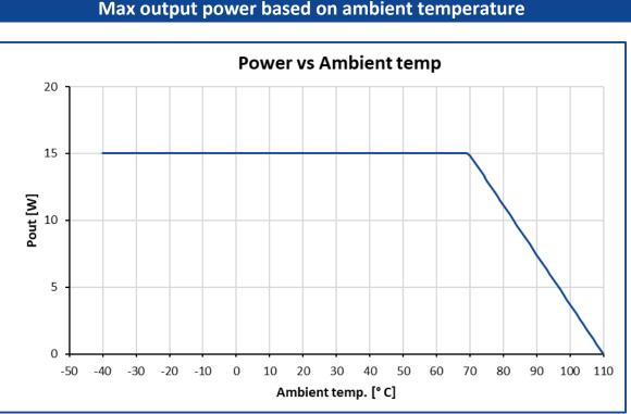
The graph is constructed for a 15 W model with 87% efficiency.
