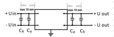
The design of the units allows their use only when mounted on a PCB. It's necessary to use certain type components. In the figure: Ck – ceramic capacitors of a certain operating voltage and of several  $\mu$ F capacity; Ce – electrolytic capacitors of a certain operating voltage and of polymer, aluminum or tantalum type of tens to
