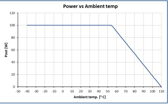
The graph is constructed for a 100 W model with 90 % efficiency.
