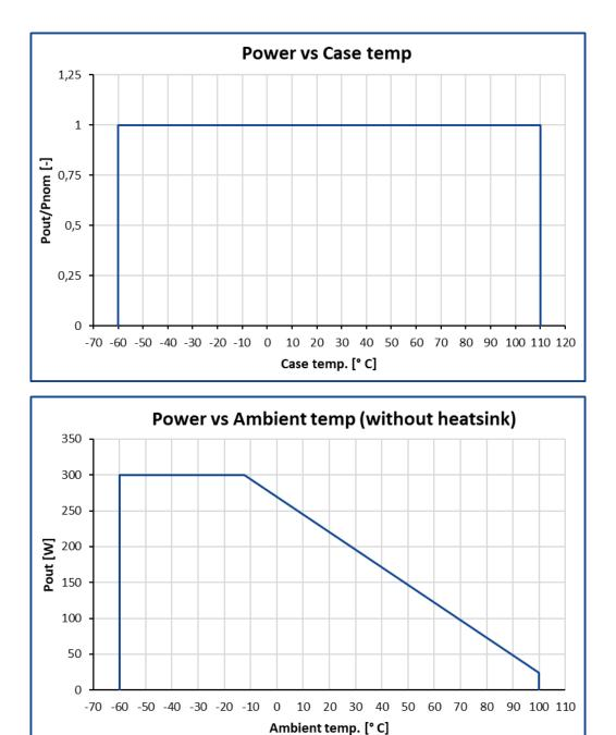
Power vs Ambient temp. graph is given for short-term use cases. To use the units without a heatsink it's mandatory to consult with the manufacturer.
