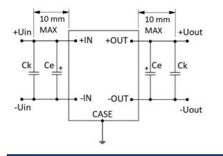
In any system application it's necessary to at least use minimal connection scheme consisting of components shown on the picture.
