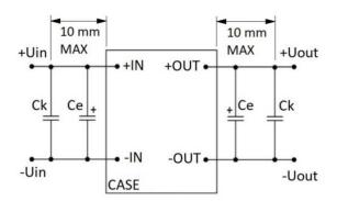
In any system application it's necessary to at least use minimal connection scheme consisting of components shown on the picture.
