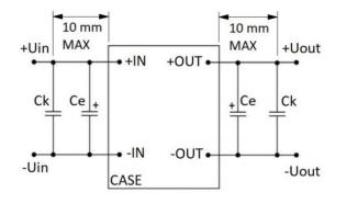
In any system application it's necessary to at least use minimal connection scheme consisting of components shown on the picture.
