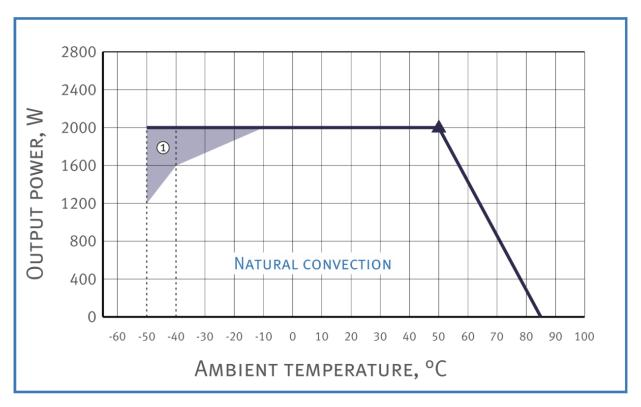
Derating curve area is in accordance with maximum case temperature of the block (+85 °C). Output power of the block must not exceed the values, limited by corresponding curve at given ambient temperature.
