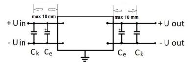
The design of the units allows their use only when mounted on a PCB. When using the units with typical connection scheme it's necessary to use certain type components. In the figure: Ck – - U out ceramic capacitors of a certain operating voltage and of several μF capacity; Ce – electrolytic capacitors of a certain operating voltage and of
