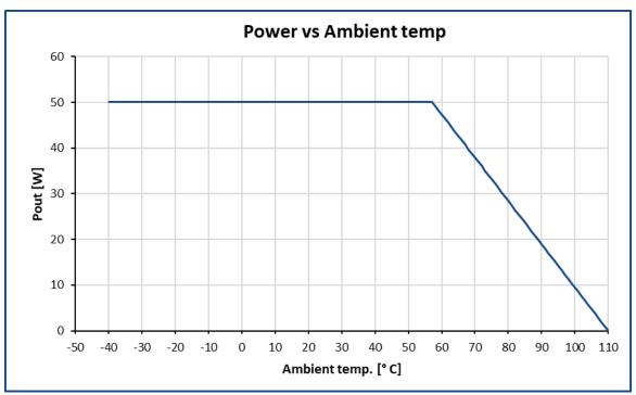
The graph is constructed for a 50 W model with 90 % efficiency.
