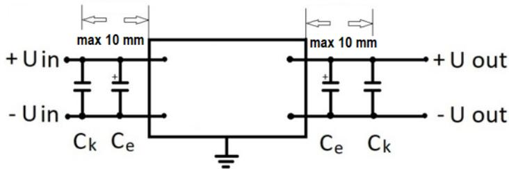
The design of the units allows their use only when mounted on a PCB. When using the units with typical connection scheme it's necessary to use certain type components. In the figure: Ck – ceramic capacitors of a certain operating voltage and of several  $\mu\text{F}$  capacity; Ce – electrolytic capacitors of a certain operating voltage and of
