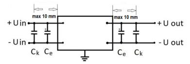
The design of the units allows their use only when mounted on a PCB. When using the units
