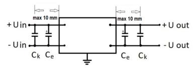
The design of the units allows their use only when mounted on a PCB. When using the units with typical connection scheme it's necessary to use certain type components. In the figure: Ck - - U out ceramic capacitors of a certain operating voltage and of several µF capacity; Ce - electrolytic capacitors of a certain operating voltage and of
