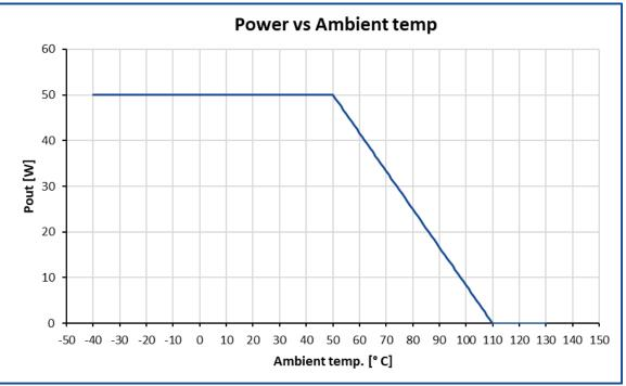
Max output power based on ambient temperature
