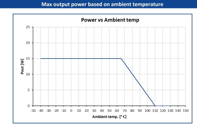
The graph is constructed for a 15 W model with 86% efficiency.
