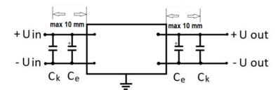
The design of the units allows their use only when mounted on a PCB. It's necessary to use certain type components. In the figure: Ck – ceramic capacitors of a certain operating voltage and of several  $\mu$ F capacity; Ce – electrolytic capacitors of a certain operating voltage and of polymer, aluminum or tantalum type of tens to
