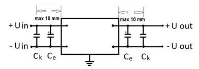
The design of the units allows their use only when mounted on a PCB. It's necessary to use + U out certain type components. In the figure: Ck – ceramic capacitors of a certain operating voltage and of several μF capacity; Ce – electrolytic capacitors of a certain operating voltage and of polymer, aluminum or tantalum type of tens to
