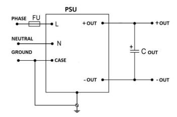
When using the units with typical connection scheme it's necessary to use certain type components.
