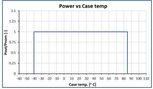
\_\_\_\_\_ Standard maximum power output based on case temperature.
