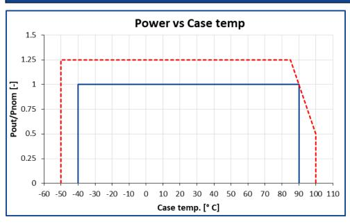
Standard maximum power output based on case temperature.
