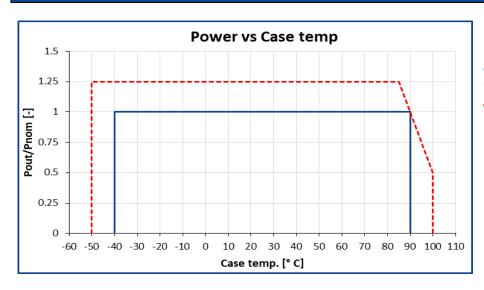
Standard maximum power output based on case temperature.
