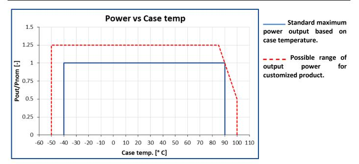
The unit must be operated on a heatsink with thermal conductive paste applied between the unit surface and a heatsink for quality contact (with thickness less than 100  $\mu$ m, of minimal thermal resistance 2 W/K.m). Mesh stencil should be used to apply paste in a pattern of 2x2 mm to 4x4 mm squares mm with 0.5-1 mm spacing between the squares. This allows paste to be evenly spread in a thin layer and excess air to escape when tightening screws during unit mounting.
